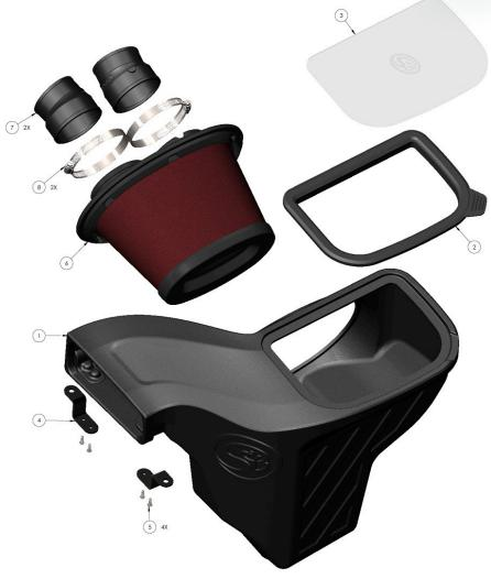
Start by loosening the hose clamps and removing the 2 bolts shown in the picture.
