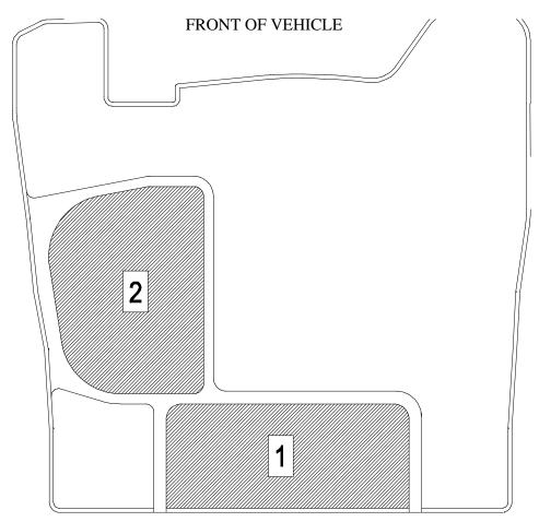
NOTE: IF YOUR VEHICLE IS EQUIPPED WITH A FACTORY CONSOLE, YOU WILL NEED TO REMOVE THE TREAD PLATE FROM AREA "1" SHOWN ABOVE BEFORE INSTALLATION. IF IT IS EQUIPPED WITH A MANUAL TRANSFER CASE SHIFTER (TRUCKS ONLY), REMOVE THE TREAD PLATE FROM AREA "2" SHOWN ABOVE. TEST FIT THE UNTRIMMED PART BEFORE TRIMMING. A UTILITY KNIFE OR HEAVY SCISSORS WORK WELL FOR TRIMMING
