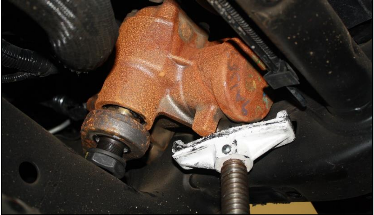
Figure 4: Support the Steering Box with a Jack
