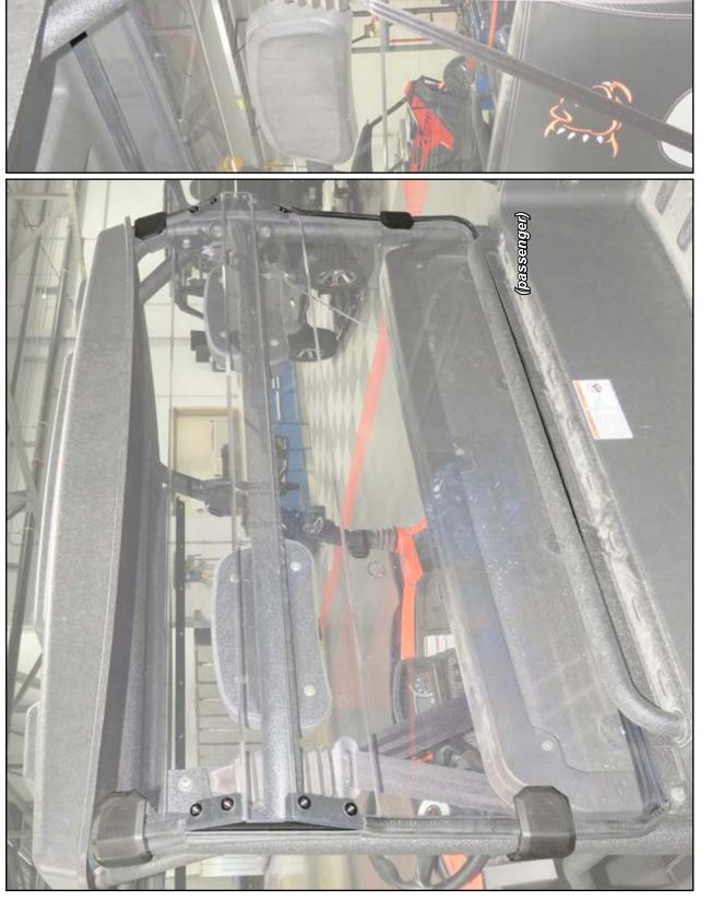
Place Windshield onto machine and secure to Cage with Clamps.
