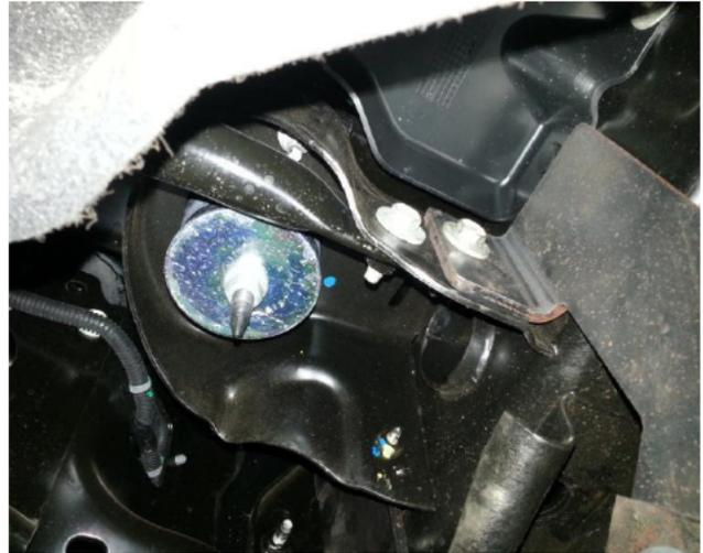
5. Install the bottom mounting bracket to the formed bracket by using two ½” x 1 ½” bolts. Allow a little movement.
