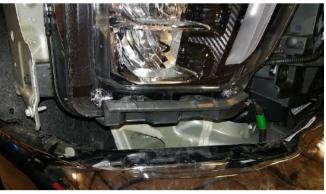
4. Remove the factory grille. Open the hood and remove the hood release latch by removing two T15 screws. Remove the ten plastic clips holding the plastic shield located above the grille.
