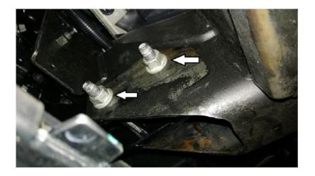
2. Install the bottom brackets by sliding the brackets from the back. The bracket mounts to the outer side of the frame. Reinsert the tow hook and use the  $5" \times 1"$  bolts to install. If no tow hooks use  $1 1" \times 1"$  bolts. You may have to trim the plastic where the brackets come through the tow hook opening.
