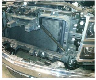
7. Remove the factory bumper by removing the two 18mm bolts from each side of the frame. They will be facing down. *See photo*
