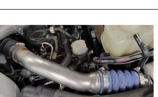
Install the air intake pipe and reconnect
