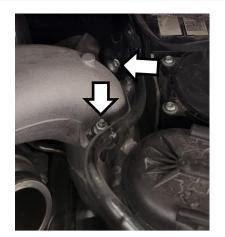
Remove the 3x bolts and turbocharger heat shield.
