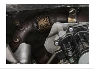
Connect the turbocharger actuator electrical connector and slide cover into place.
