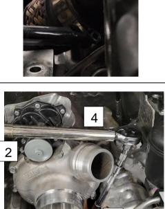
Reinstall the turbocharger coolant return tube. Use a small amount of coolant to lubricate the O-ring and seal prior to installation.
