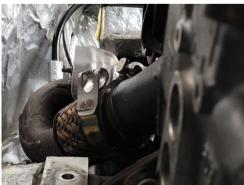
Remove the turbocharger coolant return line bolt and remove the coolant return line.
