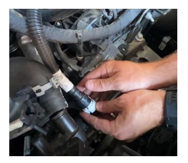
Remove the hose clamp that is attached to the turbo.
