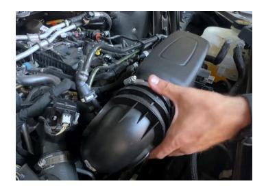
Remove the fresh air duct from the airbox then remove the airbox from the vehicle.
