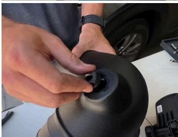
Install the grommet for the IAT sensor into the intake tube.
