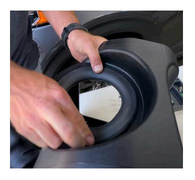
No you can decide if you wish to install the box plug. In excessively hot climates, we recommend installing the box plug.
