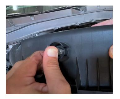
Squeeze the constant tension clamp and remove the hose from the intake tube.
