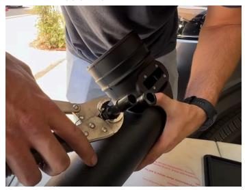
Install the gasket under the fitting plate and install onto the intake tube.
