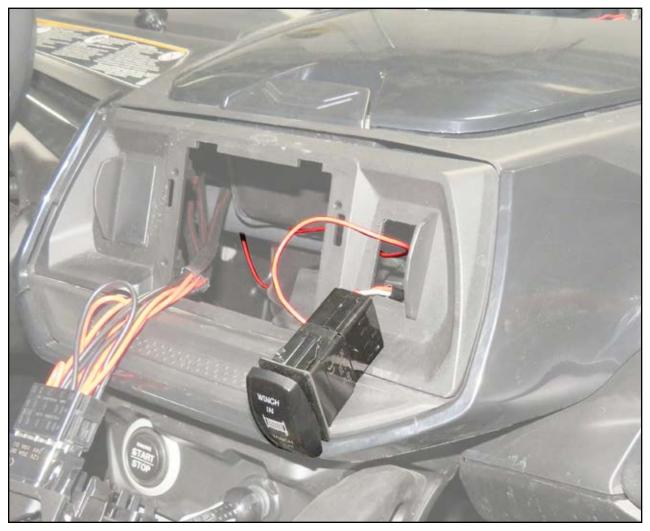
Before drilling any holes, check behind area to be drilled for any interference.
