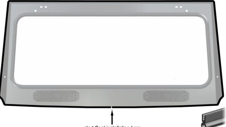
Install Seal around perimeter of Windshield as shown.
