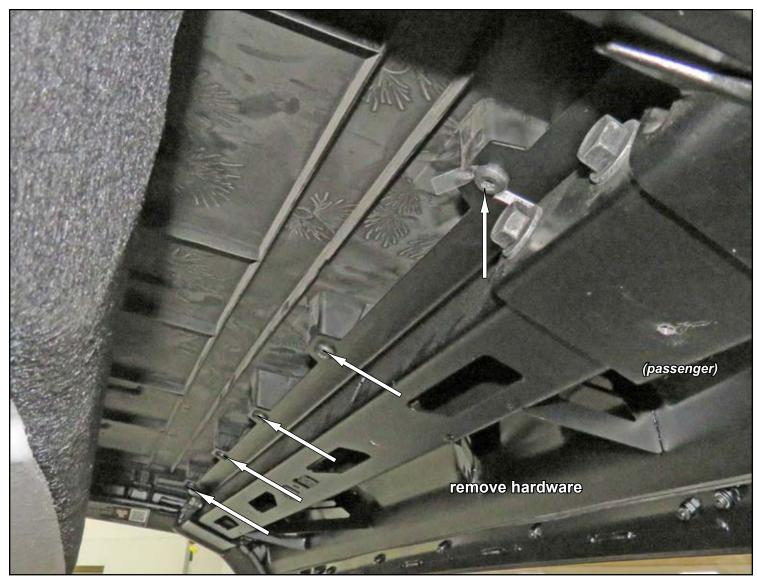
reinstall components and secure Roof after Windshield installation is complete
