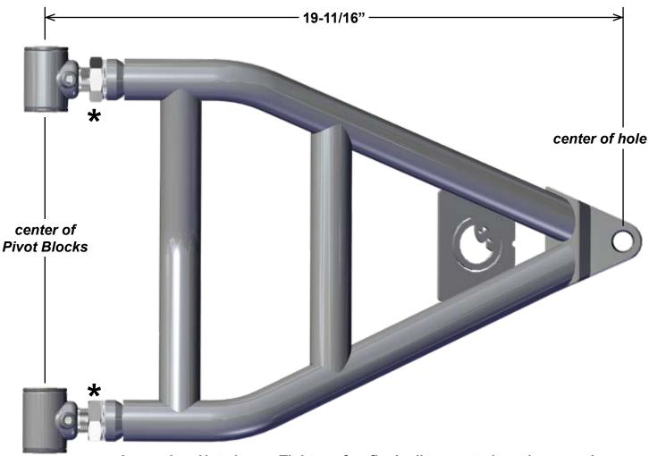
\*Leave Jam Nuts loose. Tighten after final adjustments have been made.
