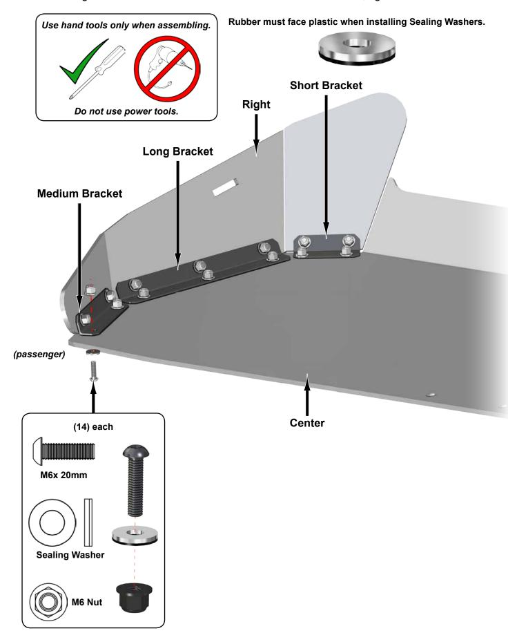
To ease installation, soak Seals in hot water before cutting or installing to increase flexibility.
