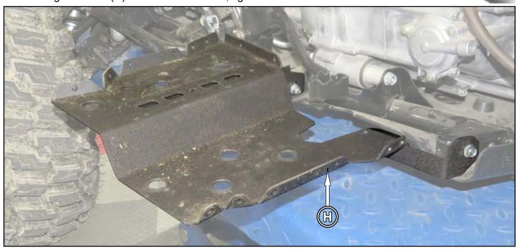
Stook - Install Front Right (B) to body and Right Bottom (H) with M6 Nut Body 3x - Spacer (m) M6 x 20mm hardware shown; tighten. 3× M6 x 16mm 2X - Install Rear Right (D) to body and Right Bottom (H) with M6 x 20mm 3x - Spacer M6 x 16mm hardware shown; tighten. š Body M6 Nut IN-FTW-H-RUBi
