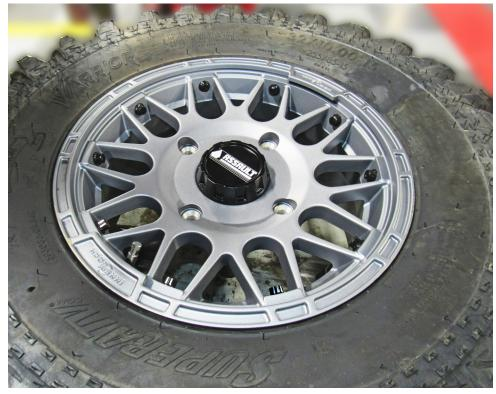
NOTE: All Bead Retention Pins to be flush with lip, and Max Torque should not exceed 30ft.lbs!
