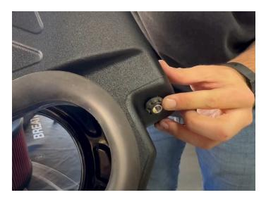
Install the S&B airbox into the truck
