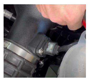
Reinstall the MAF connector to the sensor.
