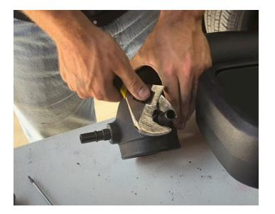
Install the coupler onto the intake tube with the hose clamps loose.
