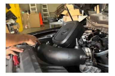
Reconnect the quick connect fittings and tighten the hose clamps.
