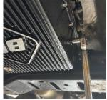
Fill the transmission through the transmission fluid filler tube with MOPAR<sup>®</sup> ASRC ATF or Mobil ATF 3309, add approximately:
