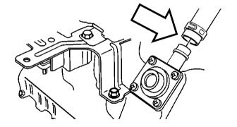
Remove the fuel injection control module from the passenger side valve cover.
