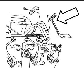
Remove the PCV hose and clamp from the driver and passenger side valve cover.
