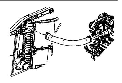
Remove air inlet and outlet hose, and battery junction box positive cable.
