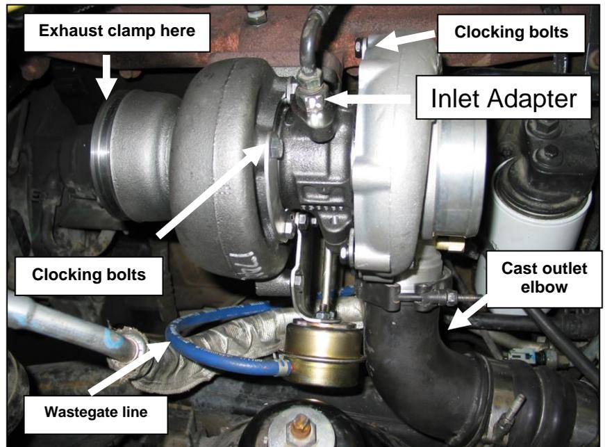
Ensure the orange o-ring is in place and use the factory v-band clamp to connect to compressor housing to the intercooler elbow and tube. Adjustment of the first intercooler boot may be required for a proper fit.
