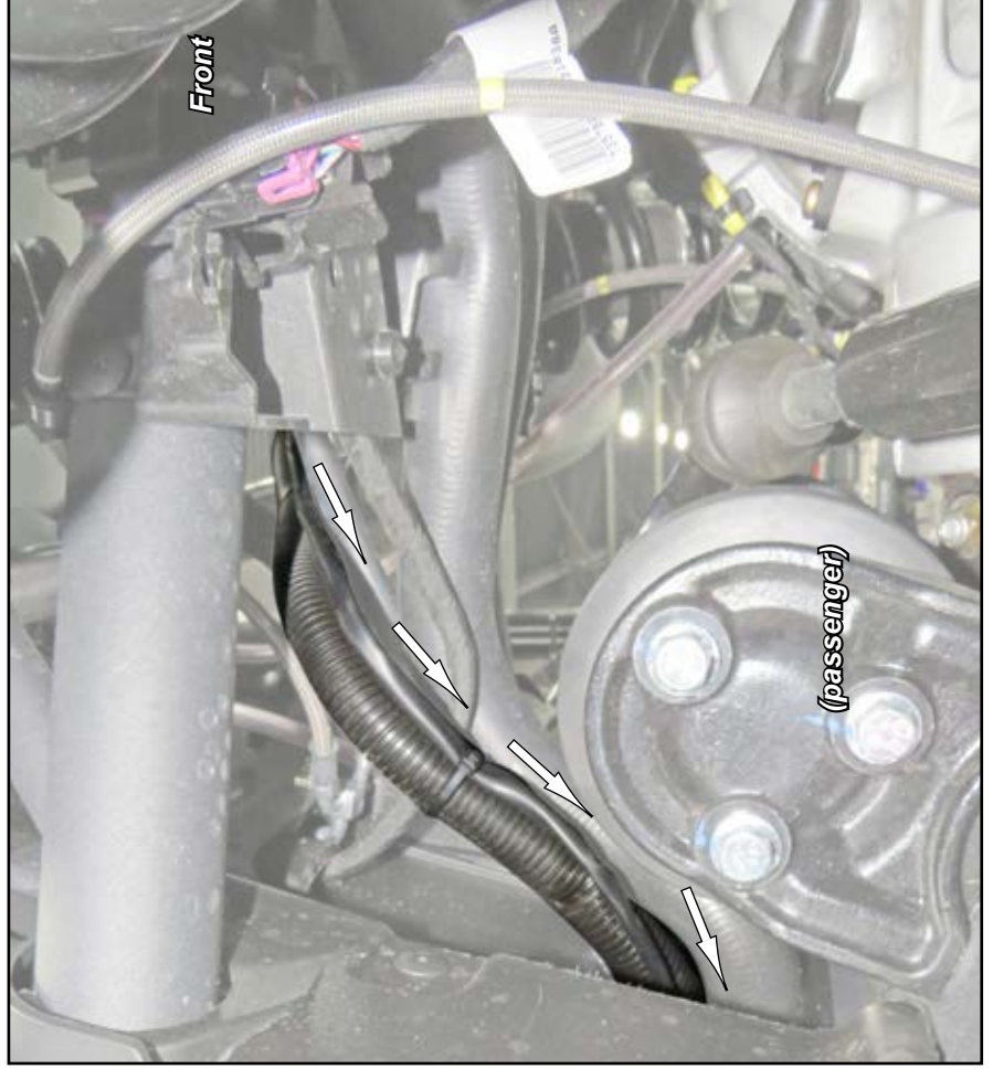
- Route Harnesses through Firewall.
