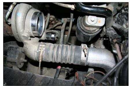
Disconnect the turbo oil supply and the turbo oil drain.
