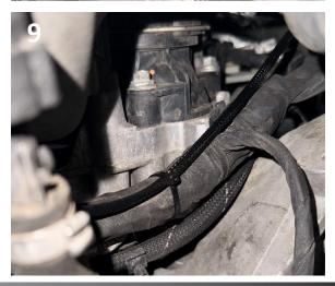
**STEP 9:** Connect the end of the harness to the alternator. Use another zip tie to retain the signal wire as shown.
