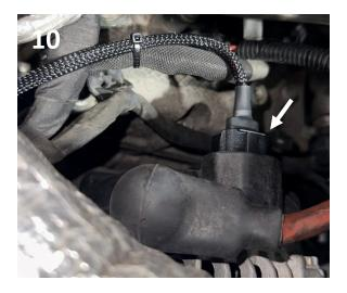
**STEP 10:** Reinstall the air intake tube, the upper half of the air filter box, and reconnect the MAF sensor.
