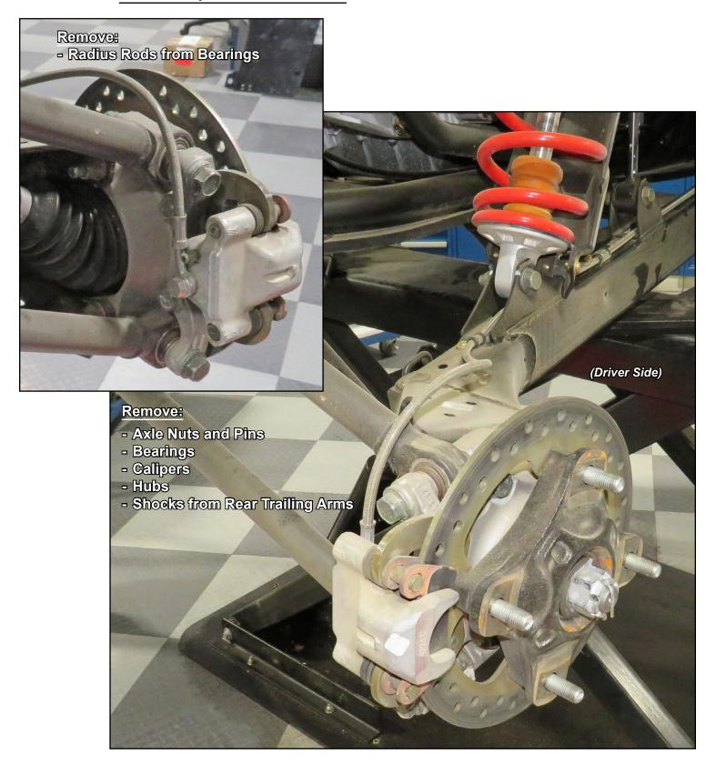
Rear Components Removal continued: Keep all components removed from machine.
