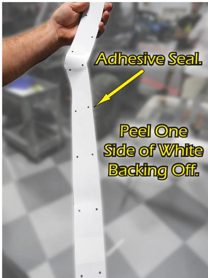
Apply Adhesive Seal To Each Metal Bracket on Top Side As Shown
