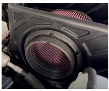
Install the coupler onto the intake tube with the hose clamps loosely installed. Line up the tap on the tube with the cutout in the filter.
