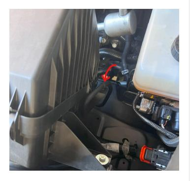
Lift the entire airbox/tube out of the vehicle.
