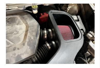
Tighten down both hose clamps on the tubes, then reinstall the two screws you remove earlier.
