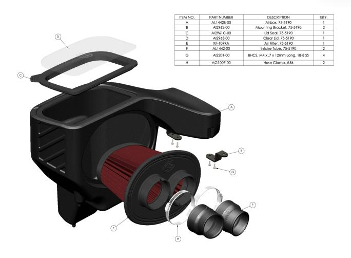
Start by loosening the hose clamps and removing the 2 bolts shown in the picture.
