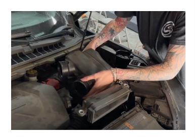
Install the S&B air filter into the S&B airbox. Then attach the hose clamps onto the flanges.
