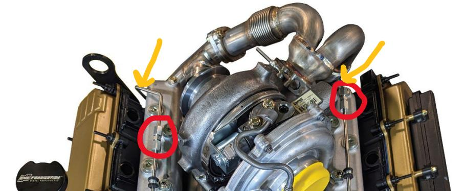
15. Install the fuel manifold/bracket assembly, only finger tight the nuts and bolts so you can align the fuel lines properly. \*\*See fuel line alignment pictures at the end of the install instructions\*\*. When aligned correctly, the tube nut should thread on without using a wrench.
