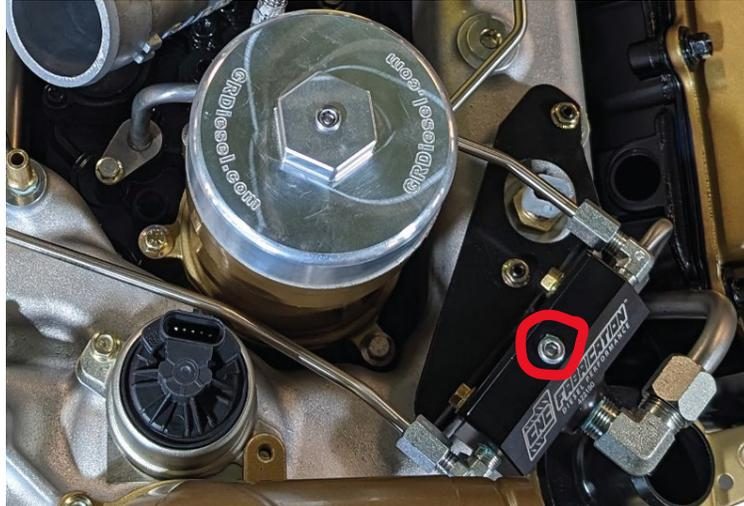
27. Remove the 1/8th inch allen head plug and apply fuel grade thread sealant to the threads and re-install the plug. If you have a fuel pressure sensor, install the sensor with the same type of sealant in place of the plug.
