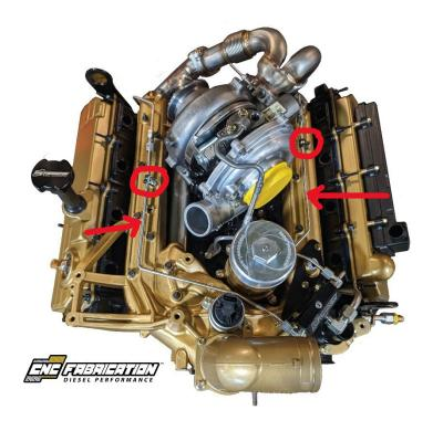
18. Remove the driver front "engine removal eyelet". This is NOT absolutely necessary, but will make it easier to install the CNC Fabrication ½ inch fuel supply line.
