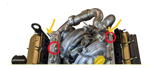
15. Install the fuel manifold/bracket assembly, only finger tight the nuts and bolts so you can align the fuel lines properly.
