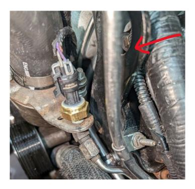
19. Feed the fuel supply hard line down behind the thermostat housing and hand thread the nut onto the fitting on the manifold block. Do not tighten yet with a wrench.
