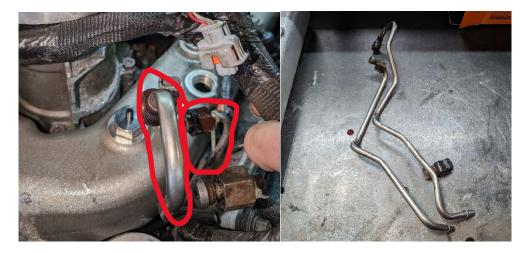
12. Remove the rear fuel rail end plugs on the back side of the driver and passenger cylinder heads. Up-pipes do NOT need to be removed but will make the job easier if you loosen the bolts at the exhaust manifold and/or the V-band clamp at the turbo. Picture below is the back of the passenger side head.
