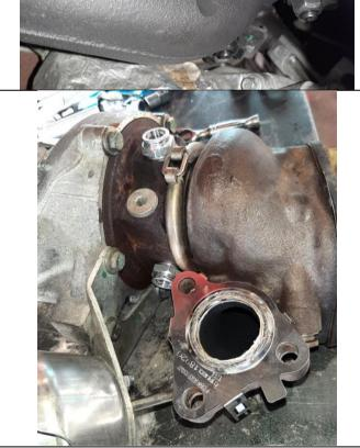
If installing a new exhaust flange gasket, do so now.
