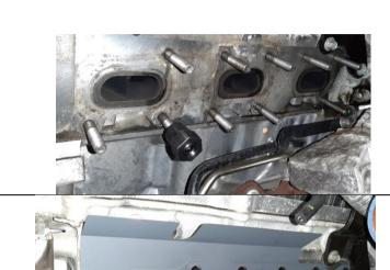
Press the exhaust manifold gaskets on (1403064/1403065). The locating tabs must be pressed on carefully to not crease or dent the gasket.
