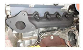
Tighten down the manifold nuts in a 3-step sequence.
