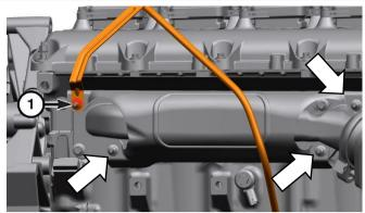
Using **10 mm & 13 mm** socket, remove the left side exhaust manifold bolts. Remove the manifold and gasket carefully
