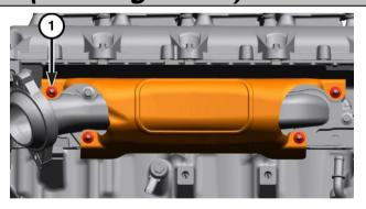
Use size **10 mm & 13 mm** socket to undo the manifold bolts.
