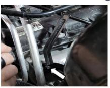
If steering shaft was disconnected, align the previously created marking and insert the upper steering shaft into lower and tighten the bolt.
