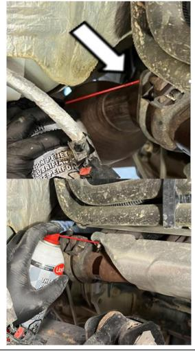
Remove the 4 flange bolts from passenger and driver side manifold to collector flange using **9/16 in** socket.
