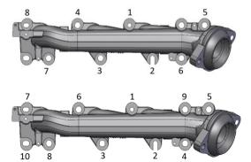
Using the provided M6 bolts (1401462), install the OEM heat shield on the new mounting locations on the BD manifold. Use size 10mm wrench.
