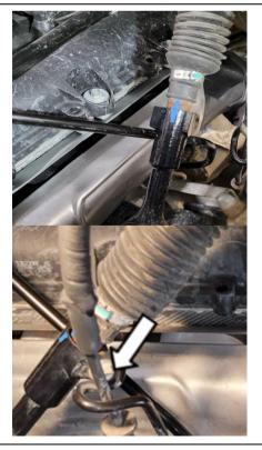
Check oil dipstick-for clearance against the hard lines after it was relocated.
