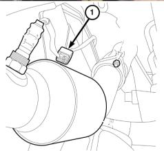
Using a **10mm** socket, remove the four heat shield nuts, and carefully remove heat shield. It will be reused.
