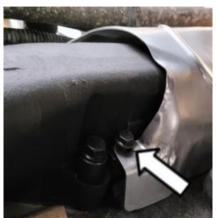
On the driver side manifold, install the dipstick support bracket onto the new mounting location using the supplied M6 bolt.
