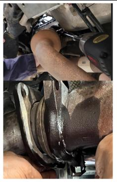
To gain more space for removal of the manifold, disconnect the mid-pipe exhaust hanger as shown.
