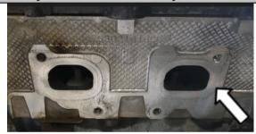
Set the manifold into position, with the corresponding gasket.
