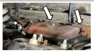
Clean and Inspect mating surfaces of exhaust manifold for flatness with a straight edge.
