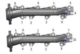
Using the provided M6 bolts, install the OEM heat shield on the new mounting locations on the BD manifold.
