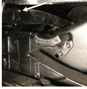
**STEP 2:** Reaching over the top side of the tank, disconnect the fuel lines and electrical connection for the OEM sending unit.
