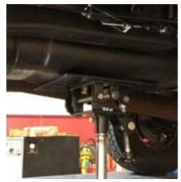
**STEP 5:** Remove 15 mm nuts that retain the fuel tank hanger brackets at the front and rear of the tank. Remove the hangers.
