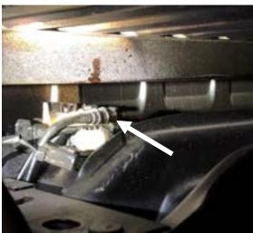
**STEP 3:** Remove the cross-member (if equipped) located at the front of the fuel tank. There will be four, 15mm bolts to remove. Some trucks will not have this cross-member.
