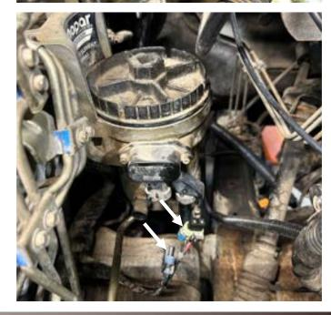
**STEP 5:** Disconnect the fuel feed line on the rearfacing side of the fuel bowl. Use a rag to capture any spilled fuel. Using a 10mm socket or wrench, remove the two bolts retaining the fuel bowl to the engine block. Remove the fuel bowl.
