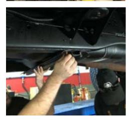
**STEP 15:** With the tank mounted in place, access the top side of the tank from the rear wheel-well and make the fuel line connections at the sending unit.
