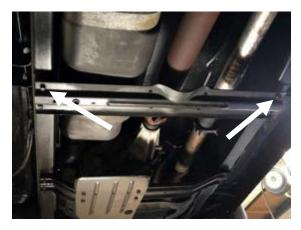
**STEP 4:** Secure the tank with a lift or jack to lower the tank down to the ground on.
