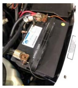
STEP 18: SWITCHED POWER Connect the switched power lead for the PowerFlo pump to the OE pump signal line, located near the starter.
