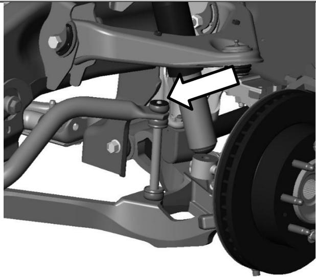
Repeat the above steps for removing the sway bar end link on the opposite side of the vehicle.
