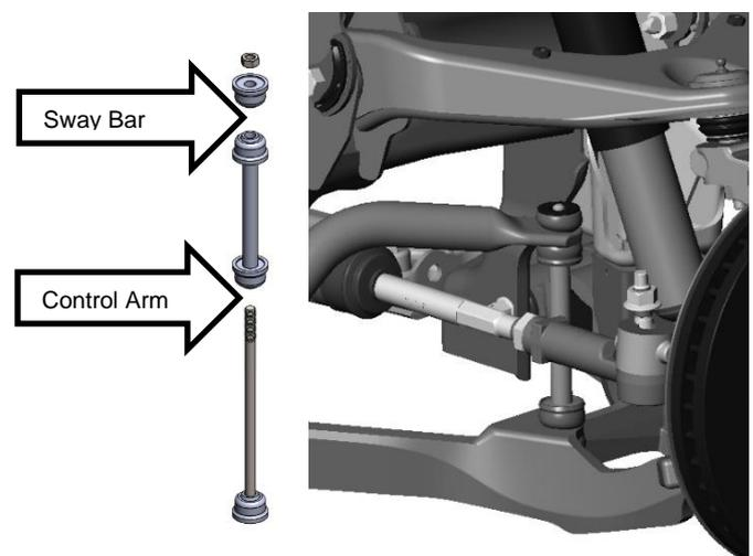
Repeat the above steps for installing the other sway bar end link on the opposite side of the vehicle.
