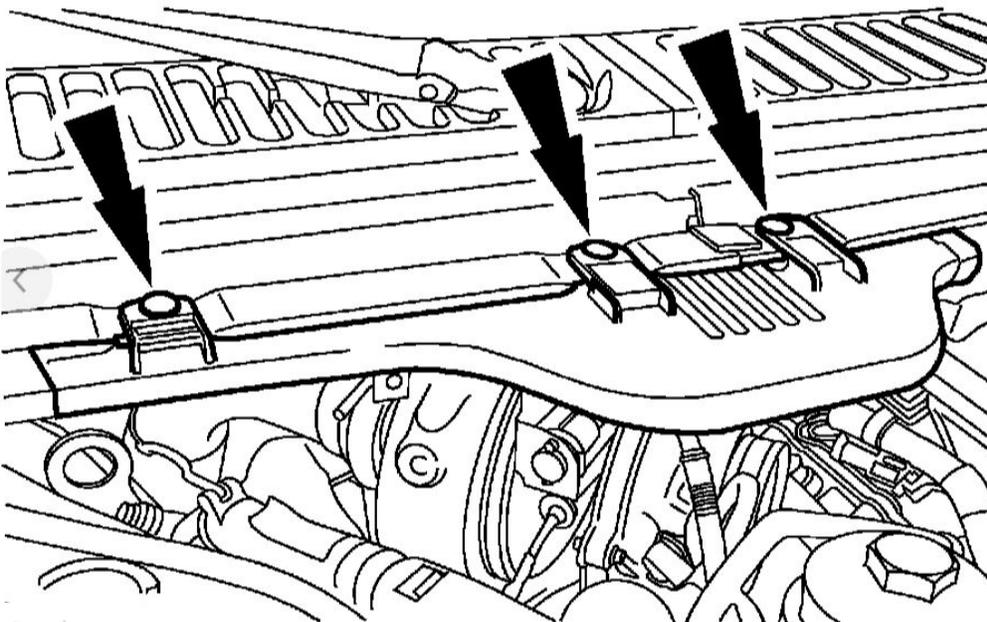
7. Disconnect the two wiring harness push pins and position aside.
