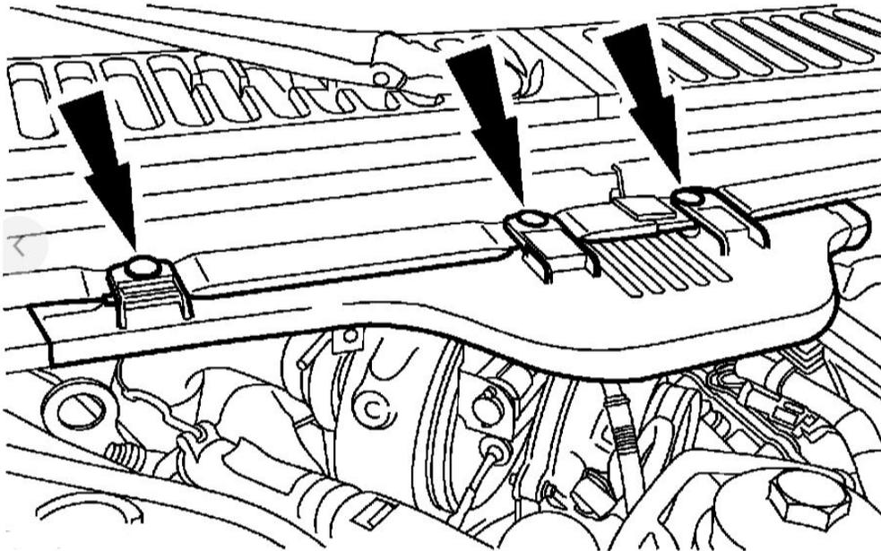
14. If there is any oil residue on charge air boot, clean both connecting ports and the inside surface of the charge air cooler pipe to prevent the pipe from blowing off. Connect the charge air cooler inlet pipe. Tighten clamp to spec.
