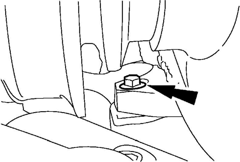
15. Remove the front mounting bolts. NOTE: Left side shown, right side similar.
