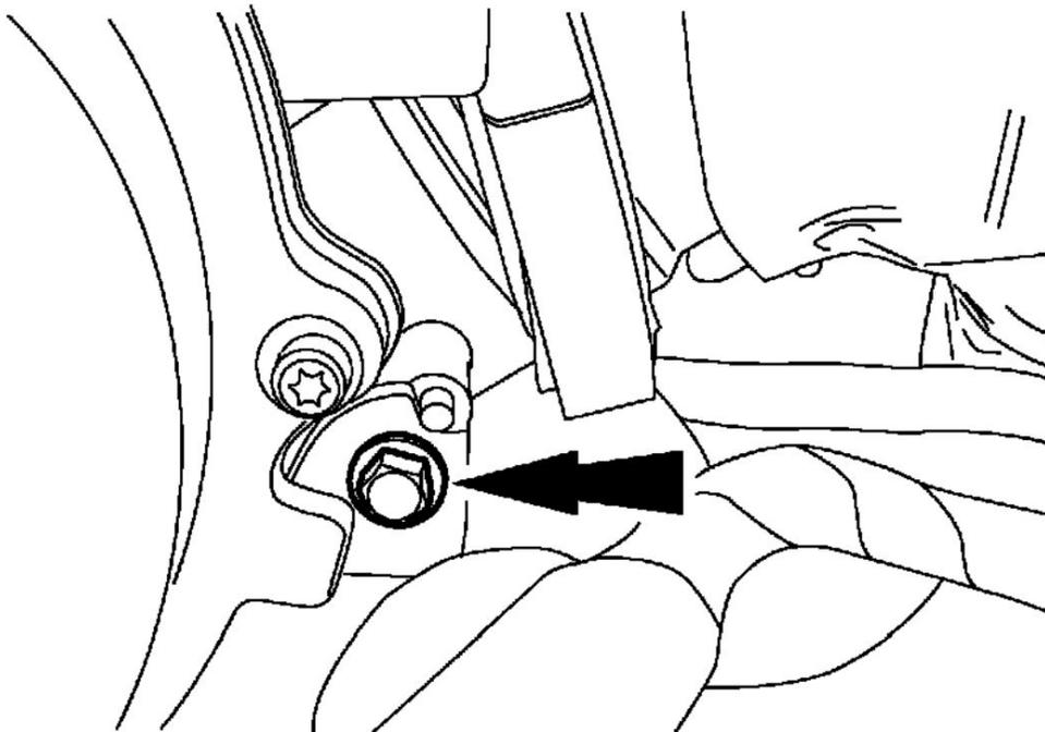
16. Position the turbocharger and remove the turbocharger drain tube. Remove and discard the drain tube O-rings
