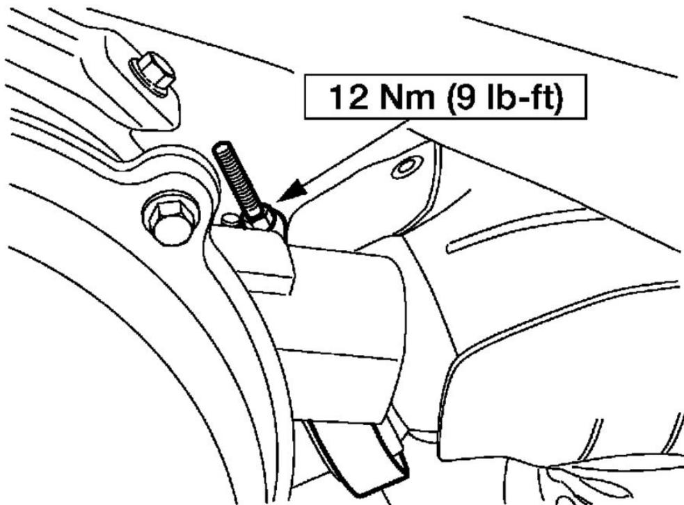
6. Install the turbocharger exhaust Mormon clamp.
