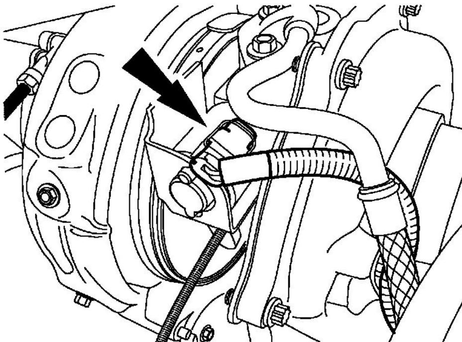
11. Position the wiring harness and connect the push pins.
