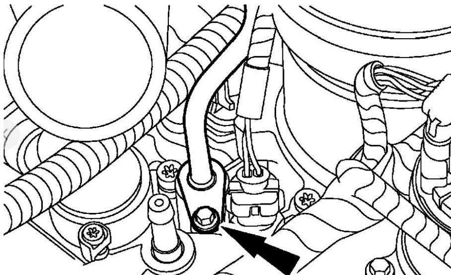
11. Remove the bolt and the wire retainer.
