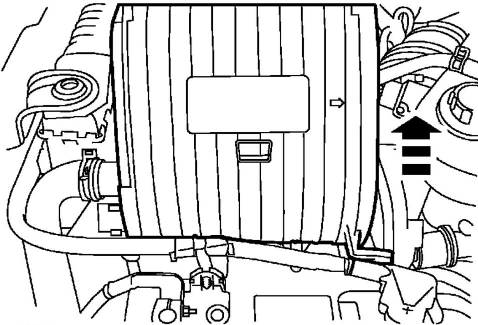
3. Disconnect the charge air cooler Inlet pipe.
