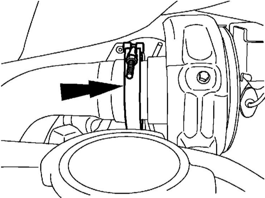
13. Remove the Mormon clamp from the turbocharger inlet up pipe.
