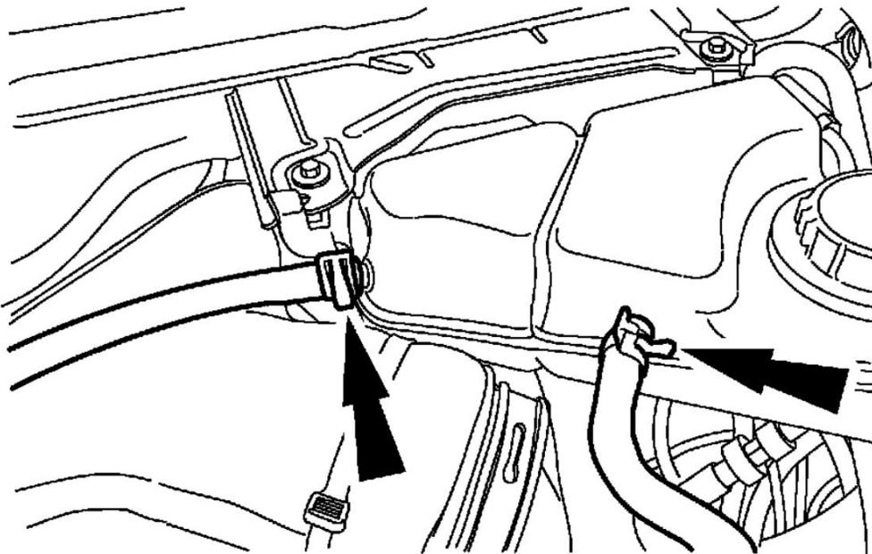
5. Remove bolts for degas bottle, move it to the side for better access
