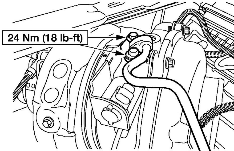
10. Connect the turbocharger variable vane hydraulic control valve electrical connector.
