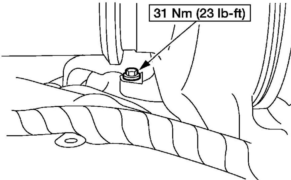
4. Install the turbocharger front mounting bolt.
