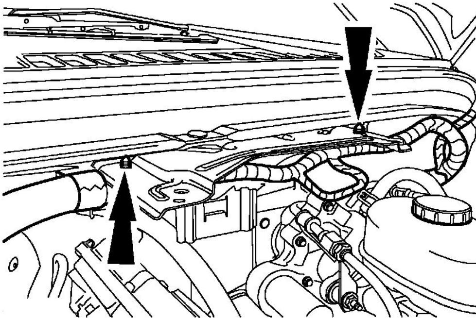
8. Disconnect the turbocharger variable vane hydraulic control valve electrical connector. (VGT Pigtail)
