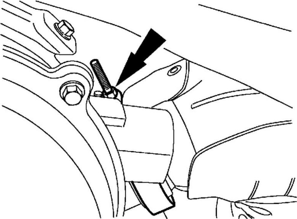
14. Remove the rear turbocharger mounting bolt.
