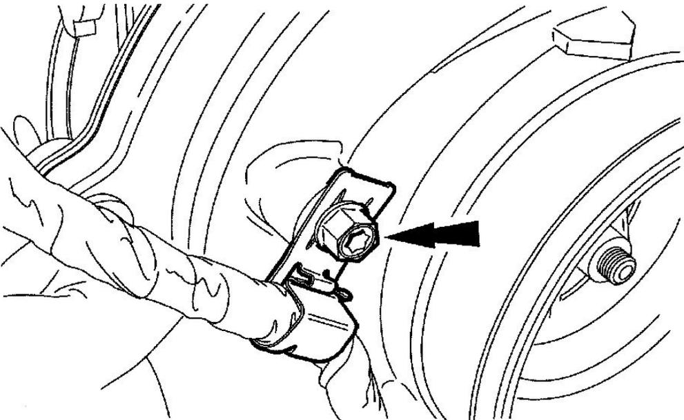
12. Remove the Mormon clamp from the turbocharger outlet / downpipe.
