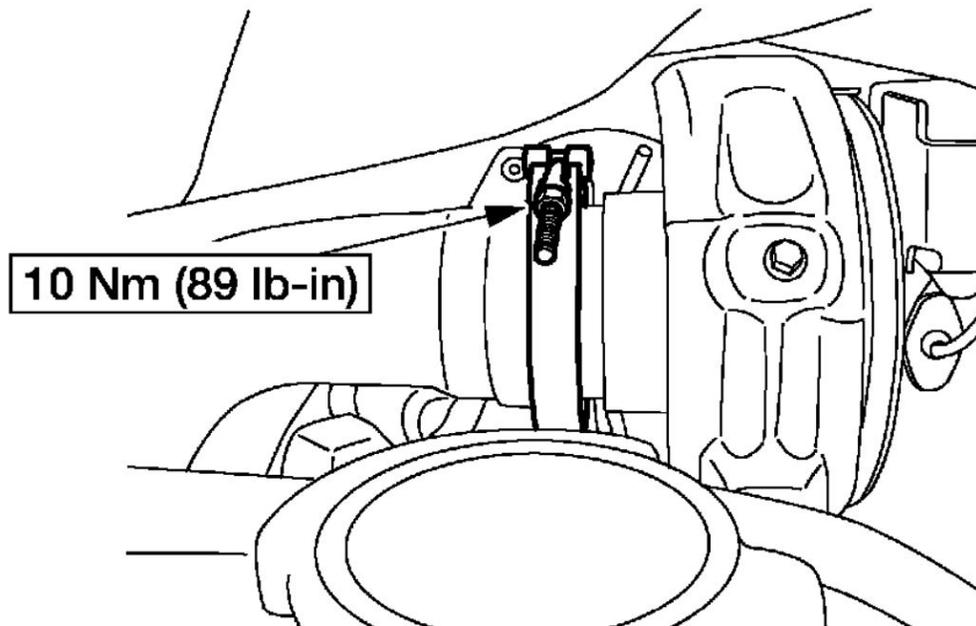
7. Install a new O-ring and apply clean engine oil. Install the oil supply tube. Position the locking bracket and install the bolt.
