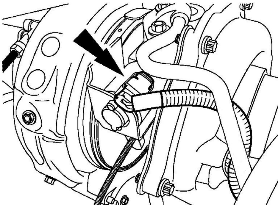
9. Remove the bolts for the oil supply tube. Remove and discard the gasket.
