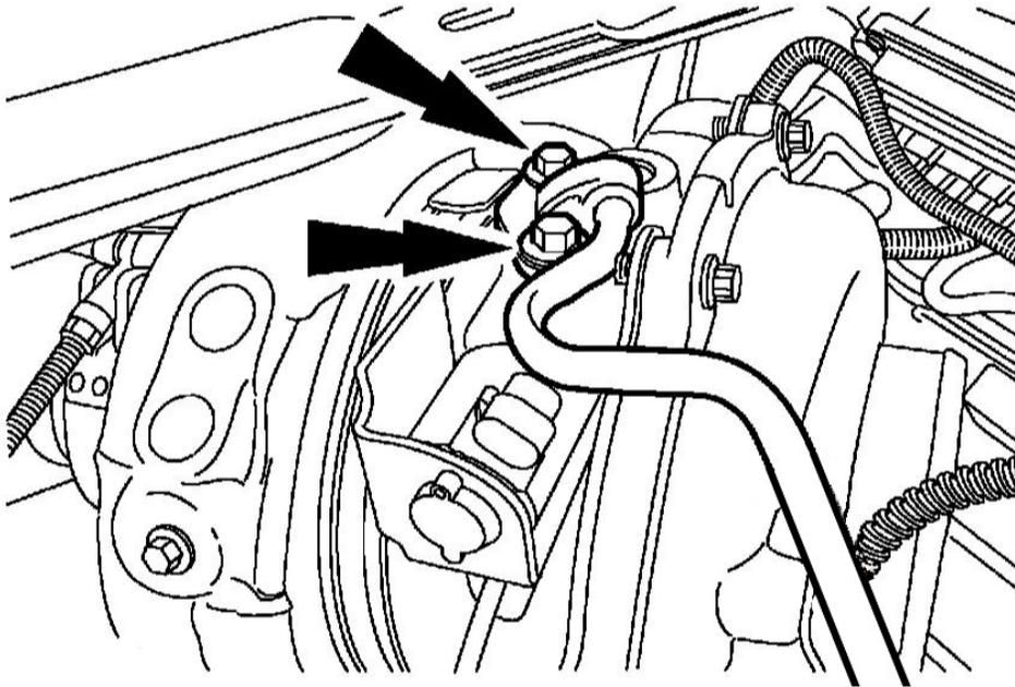
10. Remove the bolt and turbocharger oil supply tube.
