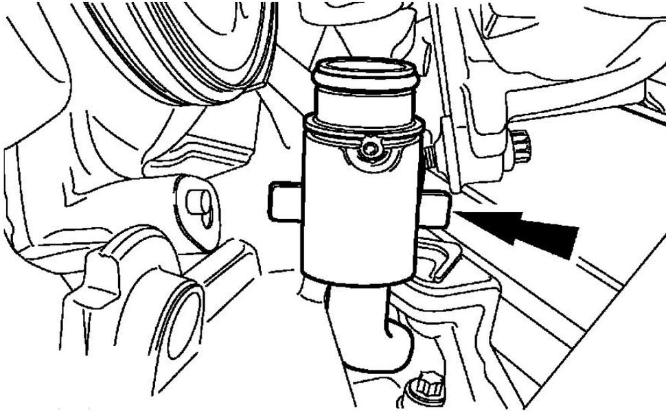
3. Install the turbocharger and the rear mounting bolt.
