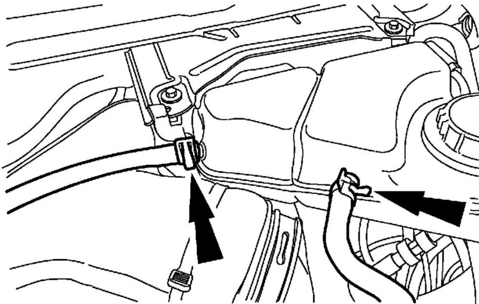
16. Install bolts and torque to spec. Top off coolant as needed.
