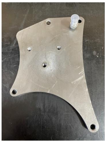
Once pedestal supply fitting is installed and new o-rings supplied are installed into the factory supply and return ports, you can rub a bit of oil on the o-rings prior to placement. The pedestal can be installed with 4 M8 X 25mm long flange bolts. Be sure no debris get into these ports while working on the vehicle. Tighten down the pedestal plate to the engine block.
