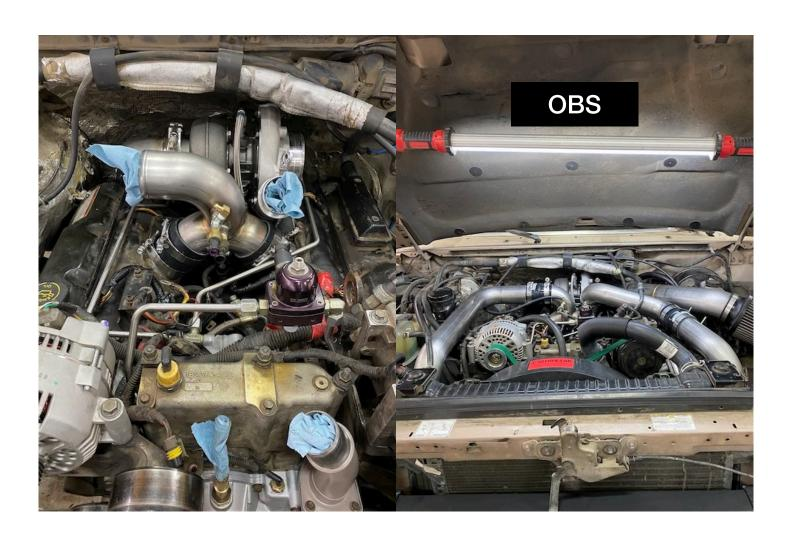
Utilizing the AFE Stage2 intakes on the SD model trucks: We have been able to run our intake pipe into an AFE air box. We removed the plastic intake pipe of the AFE kit and used our S&B 4" air filter. Or a 4-4.5 bushing can be used to maintain the AFE style of filter.
