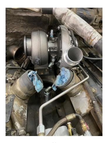
Once downpipe is fitted and installed the upper and lower sections can be tightened down. The OBS downpipe will utilize one V-band clamp and one band clamp for the mid section connection. The SD will use a 90\* elbow with a v-band at the turbine then at the upper to lower connection of the downpipe.
