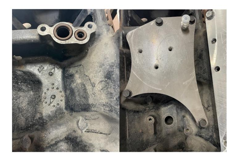
• Next install the 3/8" NPT x 10JIC 45\* fitting into the machined IDP aluminum valley drain that has the o-ring on it. Apply pipe sealant to this fitting and hand snug and no more than 2 rotations past finger tight. You can use the machined wrench flats to tighten the fitting. It does not need to be bottomed out in the flange, if you bottom the fitting out the hard line will look short and you will have to re adjust!
