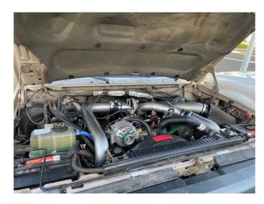
The intake pipe will have to be aligned properly for fitment of the pipes and the air filter, we recommend using our S&B filter as the "6637" style filter does not flow enough and takes up too much space by the fender well to fit correctly with the intercooler piping.
