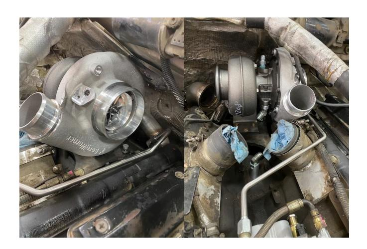
Once the drain fittings are aligned you can move to installing the oil drain line. With the center section loose on the turbine housing to allow it to rotate you can start the oil line on the bottom fitting of the turbo and rotate forward while spinning the drain assembly to rotate the line and the fittings together. This is a tricky process, but once done is a fail proof setup.
