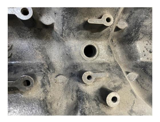
• The drain flange doesn't need to be pressed all of the way into the block. The o-ring on the cylinder will seal off the port from the weather. It can have a bit of lubricant added to the o-ring as well to help ease installation of the drain assembly into the motor. The flange stays loose and is able to be rotated around when it comes to installing the stainless turbo drain line.
