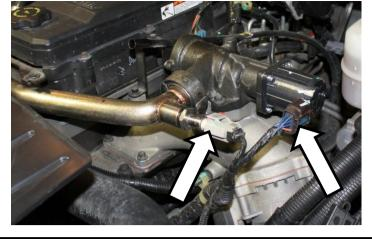
3. Loosen the EGR cross over pipe clamps (11 mm) and slide them down the pipe. Remove the bolt located at the center of the pipe, and remove the pipe from the vehicle (8mm).
