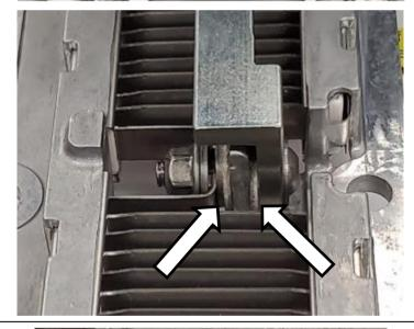
5. Install the new upper busbar assembly into the top of the grid heater.
