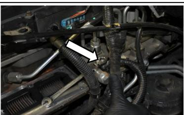
21. Remove the four bolts holding the fuel rail to the grid heater (10mm).
