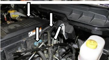
10. Reconnect the harness clips onto the fuel rail in the same location as they were removed from.
