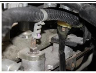
18. Disconnect CCV pressure sensor harness connector that is located at rear of the valve cover. This needs to be disconnected to allow you to coil the harness aside to access the grid heater.
