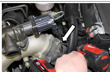
6. Pull off the harness clip from the intake horn.
