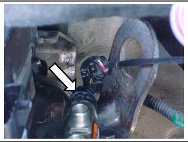
23. Remove the four remaining bolts that hold the grid heater to the engine.
