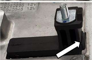
2. To remove the bottom busbar, use the included IP25 Torx Plus bit and slim 10mm wrench to remove the bolt and nut in between the heating elements. Retain the small insert that fits in the bolt hole and the flat steel washers.
