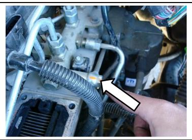
14. Remove the six injector lines starting with loosening of the fittings at the front of the fuel rail and the #1 injector (19mm). As you remove the fuel lines identify them in some way (eg. masking tape and felt pen) so they can be easily reinstalled in the same location.
