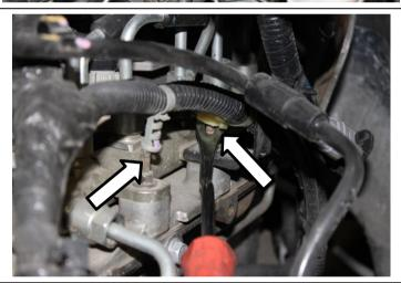
11. Reconnect the throttle valve sensor to the bottom of the intake horn.
