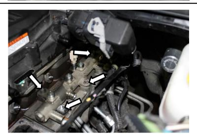
22. Disconnect the fuel rail connector from the back of the rail. The rail can now be removed from the vehicle.
