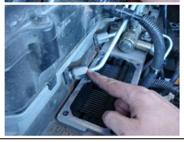
15. Disconnect the intake air temperature sensor connector from the grid heater.
