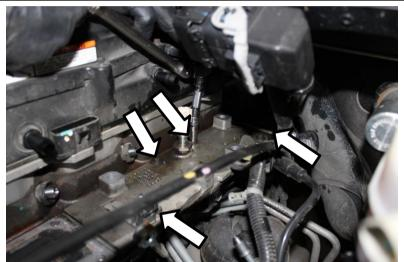
24. With the four bolts removed you may need to gently pry the grid heater from the gasket before it can be removed from the vehicle.
