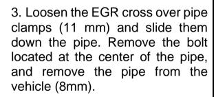
Note: When releasing the pipe from the engine there will be a loose washer on the left side. Be sure not to lose this as it will be reused.
