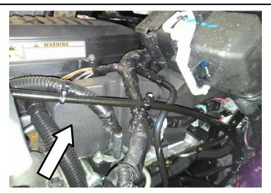
12. Loosen the fittings on the line that goes from the fuel rail to the fuel pump. Once both fittings are loose the line can be removed from the vehicle (19mm).
