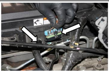
17. Using a puller tool pull out the harness clips that secure the harness to the grid heater and the other clip on the backside of the valve cover.
