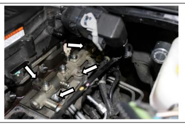
3. Reinstall the six injector lines (19mm), an easy task if previously marked for identification.
