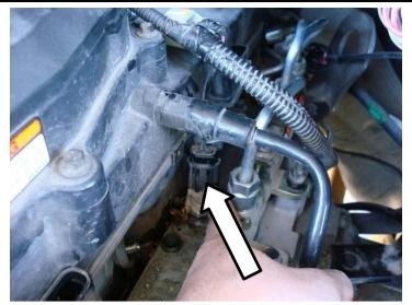
16. Disconnect the breather hose to the motor. Disconnect the two fuel line harness connectors on the side of the motor.
