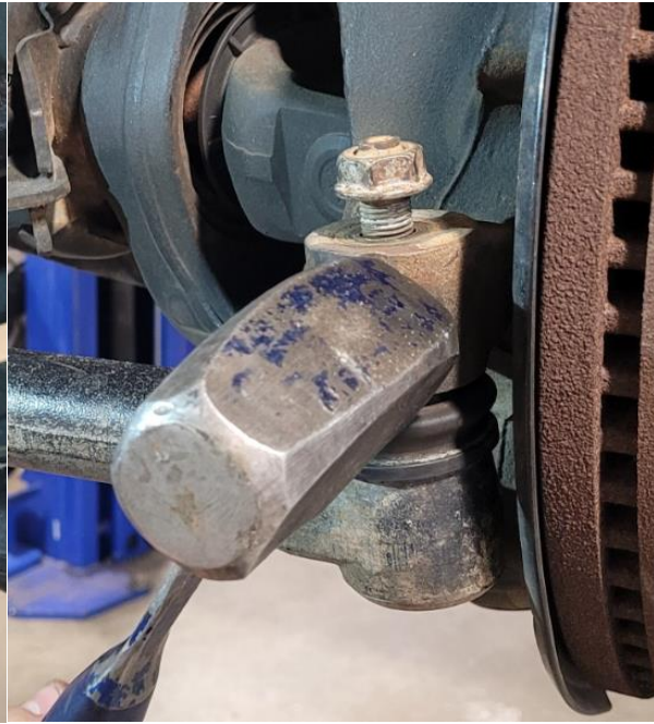
Figure 2. Separating Drivers Side
