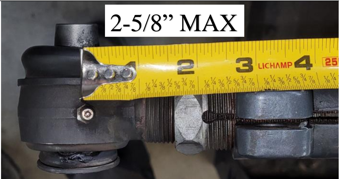
Figure 5. Double Adjuster Tie Rod End Maximum Extension.
