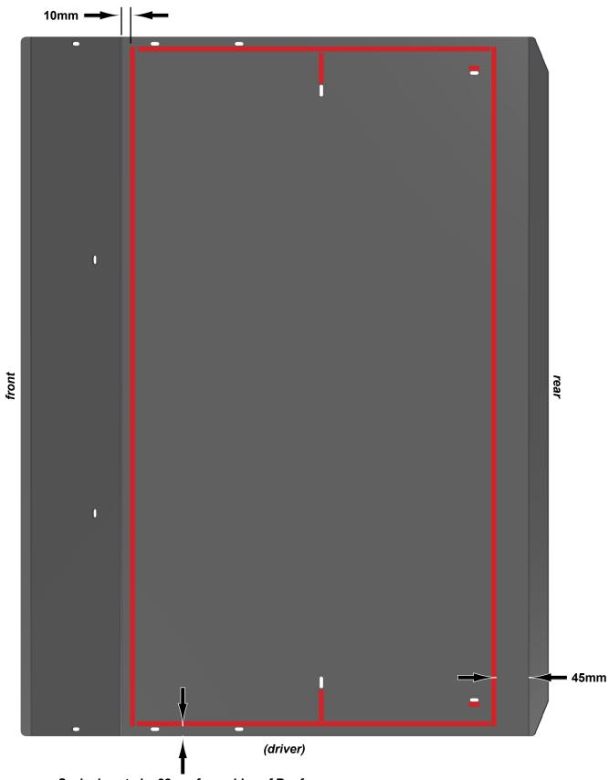
Seal edges to be 22mm from sides of Roof.
