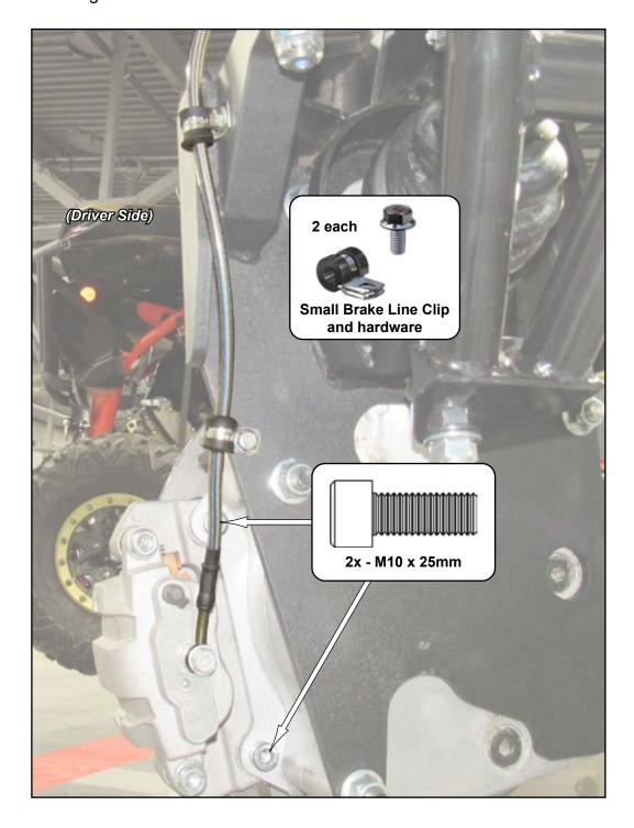
**Rear:** do not tighten hardware completely unless noted.
