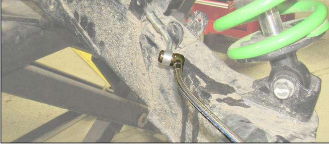
Connect Rear Brake Line Extension to Caliper.
