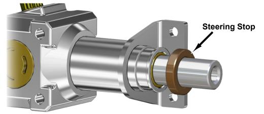
Rear Components Removal: Keep all components removed from machine.
