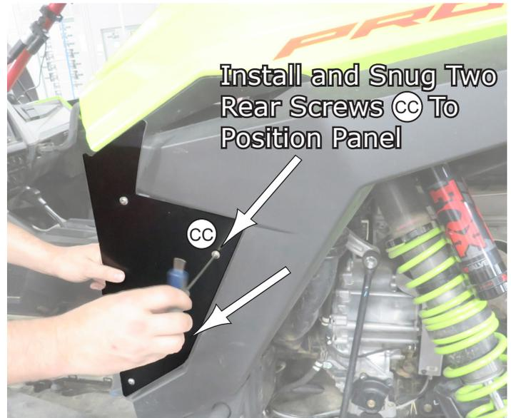
Install and Snug Two Rear Screws (CC) To Position Panel
