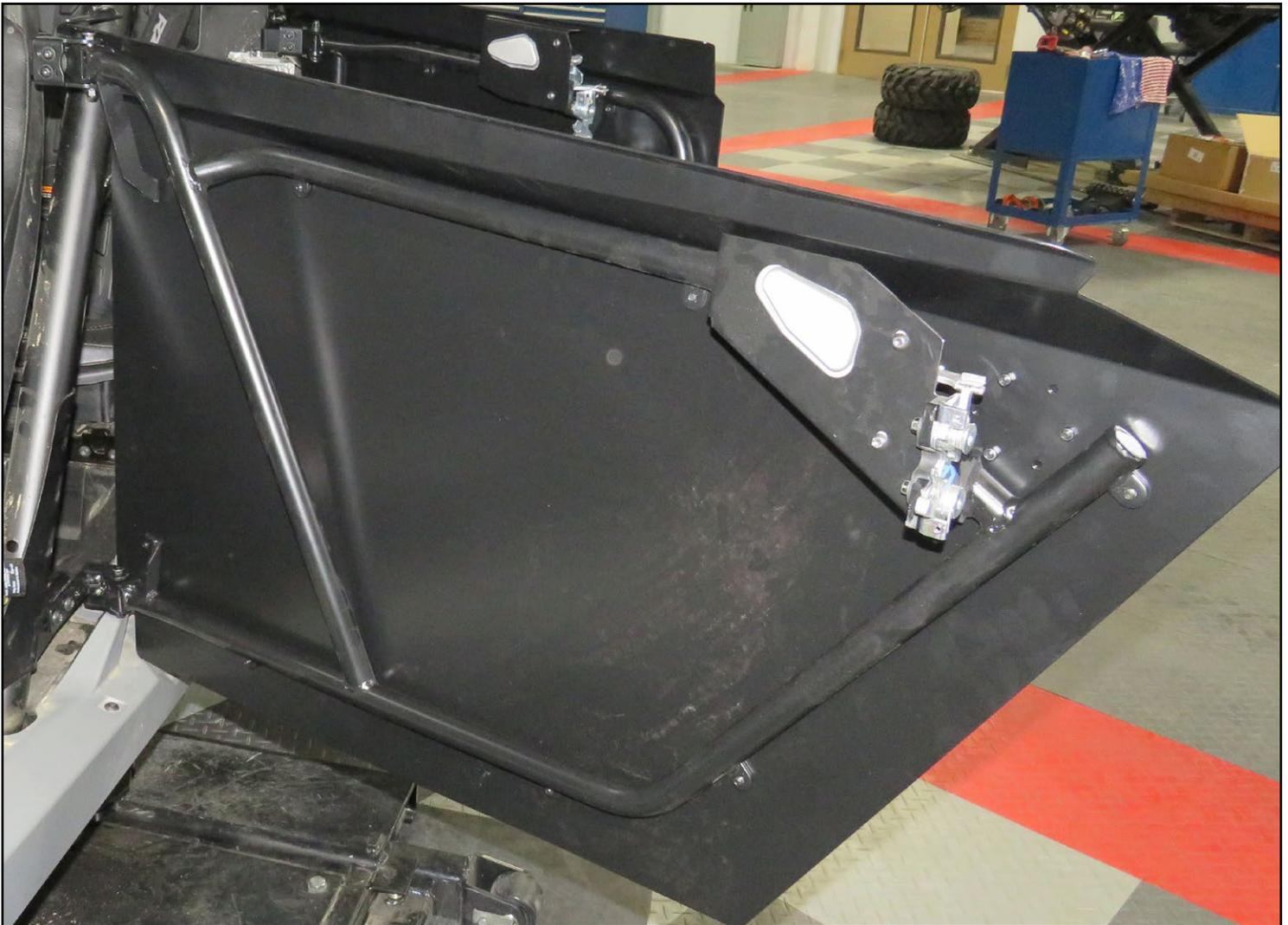
**Adjusting Doors is easier with someone inside of machine to tighten hardware and another person outside of machine to adjust Doors into place.**
