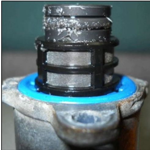
Image 2 – Example of condition from pump failure
