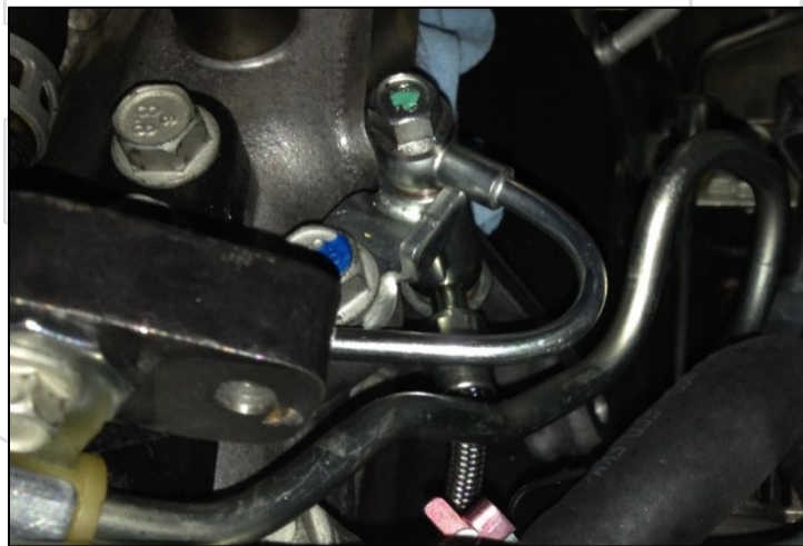
Image 10 – hydrocarbon injector line installed
