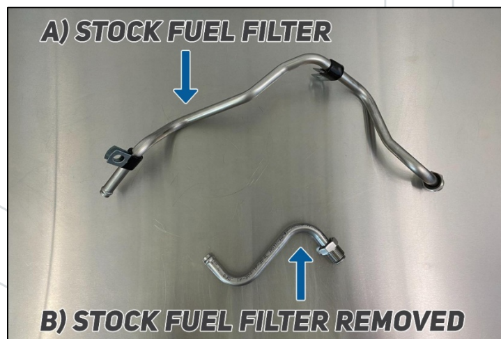
Image 8 – Line A should be used with the stock fuel filter housing. Line B should be used when the stock fuel filter housing has been removed (fuel supply hose for Cp3 is not included).
