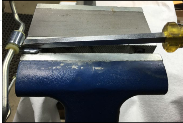
Image 7- Remove clamp from rail-to-rail cross-over HP fuel line.
