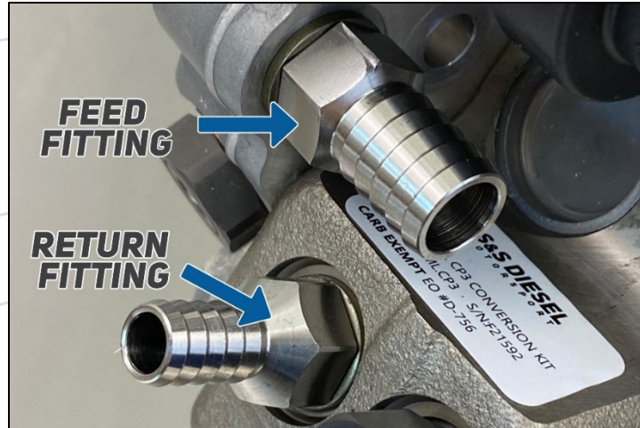
Image 4 - Large barbed fitting is the fuel feed and small barbed fitting is the fuel return
