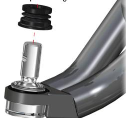
Pump in (1) shot of Grease.Ride machine and Grease again.
