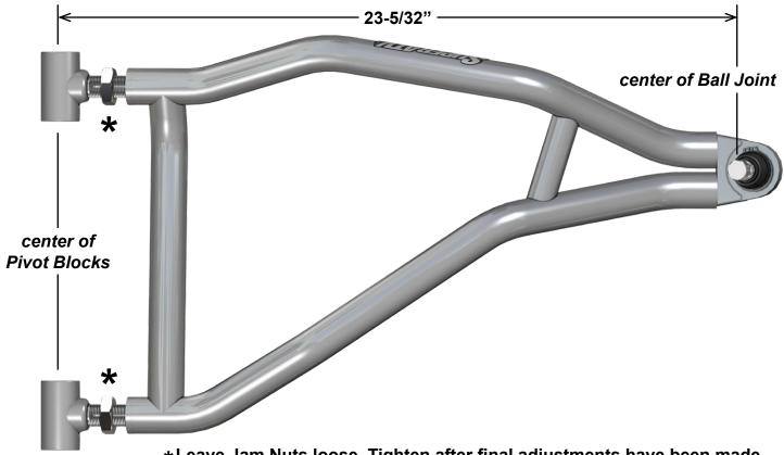
\*Leave Jam Nuts loose. Tighten after final adjustments have been made.
