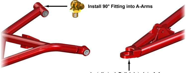
Install stock Ball Joints into A-Arms; disregard if SuperATV Ball Joints are included
