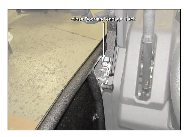
align Door to machine and tighten all hardware completely
