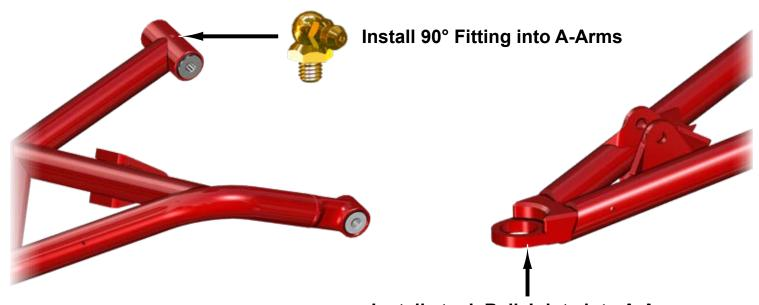
Install stock Ball Joints into A-Arms; disregard if SuperATV Ball Joints are included
