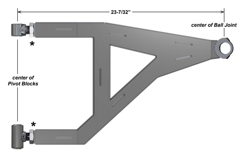
\*Leave Jam Nuts loose. Tighten after final adjustments have been made.
