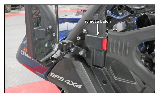
do not tighten hardware completely unless noted (driver side installation shown)
