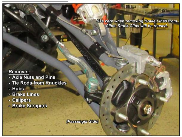
Rear Components Removal: Keep all components removed from machine.
