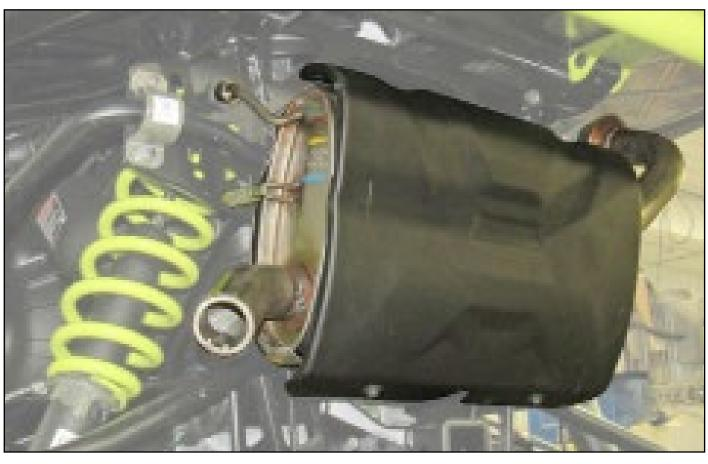
To access A-Arm hardware, Muffler must be removed if located as shown.
